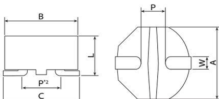
\*2 : The dimension P (the distance between terminals) shall be the shortest distance between the land and grounding surface.
